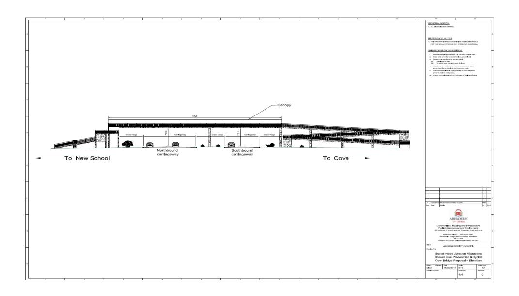
A proposed design layout and elevation drawing for the pedestrian overbridge is provided above. This illustrates the proposed footprint of the scheme. It is assumed the bridge clearance over the A class road would be 7 metres.
